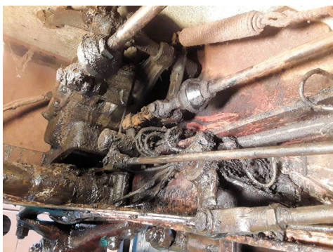
The underside driver's cab cleaning in progress on Cardiff 262.
