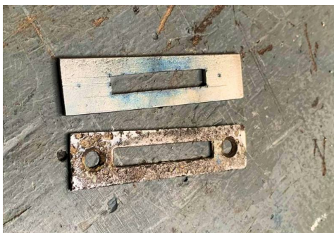
The budget lock receiver plates, both new and the old, which was used as pattern.
